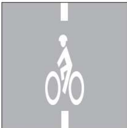
Bike detector pavement marking MUTCD Fig. 9C-7
