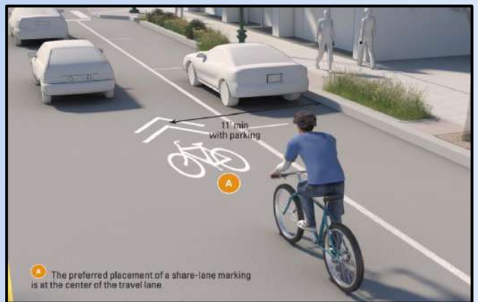
Source: NJDOT Complete Streets Design Guide
